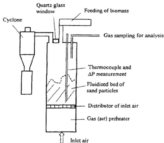
Fig. 1. The experimental unit for biomass burning and agglomeration
