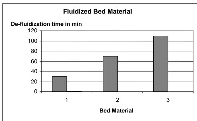
Fig. 3. Influence of fluidized bed material on defluidization time (t = 850°C)
