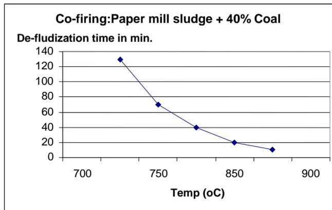
Fig. 4. co-firing paper mill sludge with 40 mass % of coal
