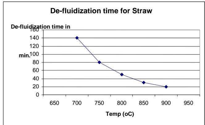
Fig. 2. Influence of FBC temperature on time needed for
